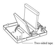
6 Tape the cable to the battery body, and put the battery in a plastic bag, etc.
